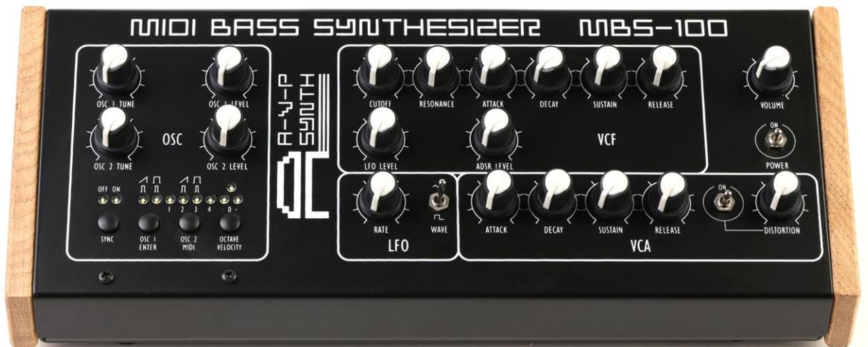
**MBS-100** - is a monophonic bass synthesizer inspired by synthesizers produced in the soviet era times while having the flexibility, MIDI control and compact package of the 21<sup>st</sup> century. It has 19 knobs, 3 switches and 4 buttons with which you can control the parameters of the sound and MIDI.
